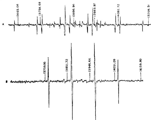
Figure 1. (a) The esr spectrum of ethyl radical from the photolysis of *t*-butyl perpropionate at  $-90^\circ$ . (b) The esr spectrum of methyl radical from the photolysis of *t*-amyl peracetate at  $-90^\circ$ .
