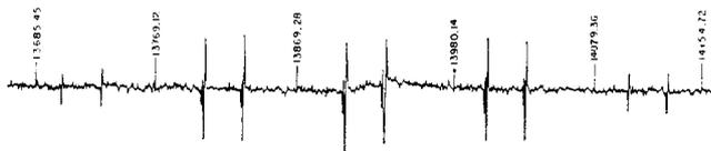
Figure 3. The esr spectrum of cyclopropyl radical from the photolysis of *t*-butyl per cyclopropanecarboxylate at  $-100^\circ$ . The proton nmr field markers are in kilohertz. Note broad-line absorption at *ca.*  $g = 2.00$ .
